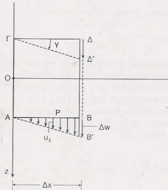
$$[\epsilon] = \begin{bmatrix} 0 & \frac{1}{2} \gamma \\ \frac{1}{2} \gamma & 0 \end{bmatrix}, \quad [\omega] = \begin{bmatrix} 0 & -\frac{1}{2} \gamma \\ \frac{1}{2} \gamma & 0 \end{bmatrix} \Rightarrow \omega = \frac{1}{2} \gamma$$
