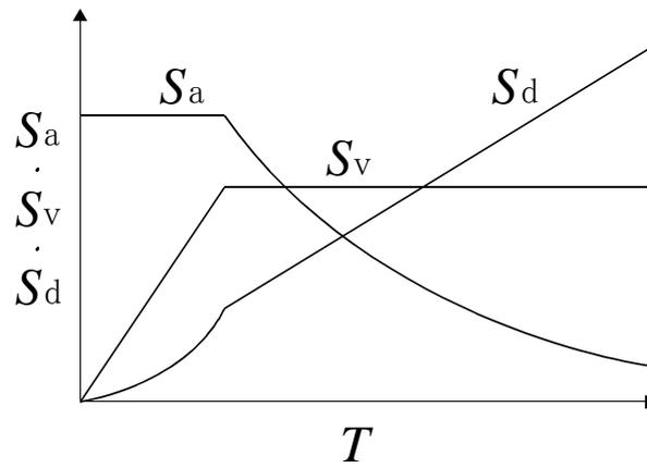
Fig.2.4.4 Typical characteristics of response spectra
