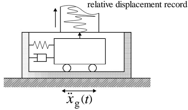
**Fig.2.3.4** Scheme of a seismometer
