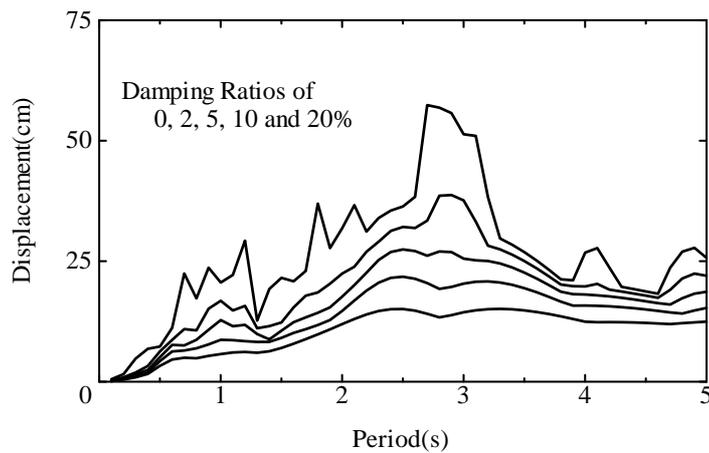
**Fig.2.4.3(c)** Displacement response spectrum (El Centro 1940 NS)
