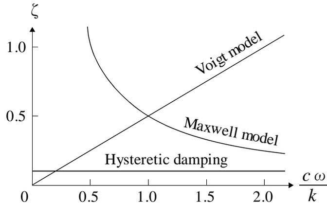
Fig.3.5.4 Frequency dependency of damping factor for each model
