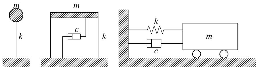
**Fig.2.1** Analytical models of single degree of freedom (SDOF) systems
