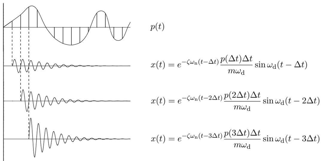
**Fig.2.4.1** Convolution integral
