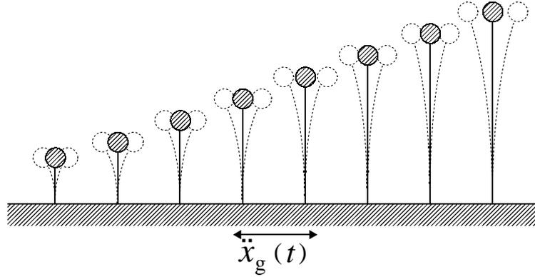
**Fig.2.4.2** Scheme of response spectrum
