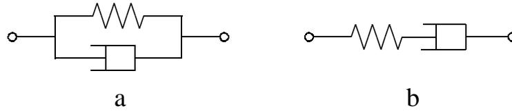
**Fig.3.5.1** (a) Damping for Voigt model and (b) Maxwell model
