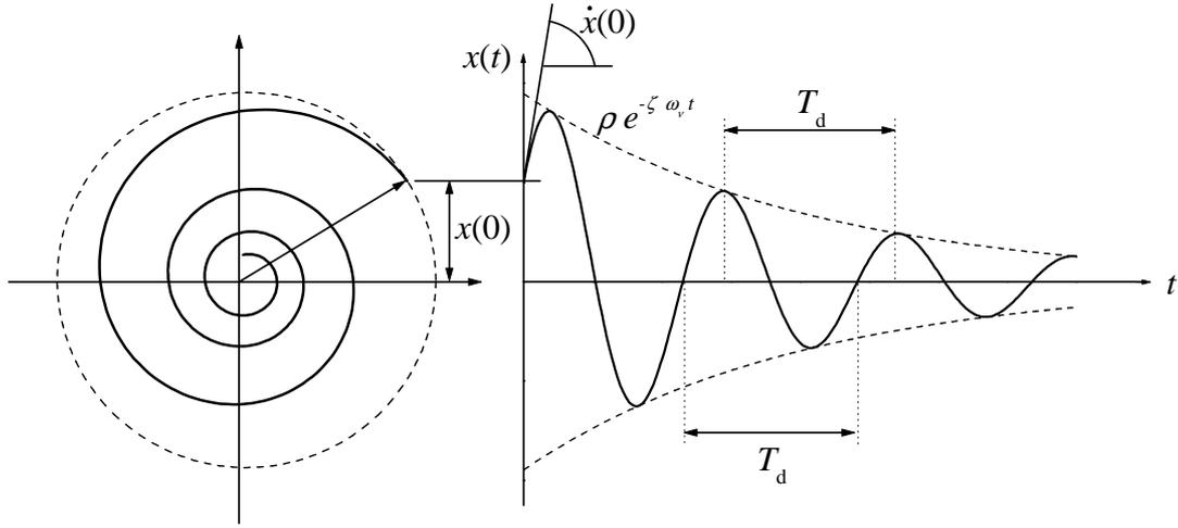
**Fig.2.2.6** Free vibration response of an underdamped system
