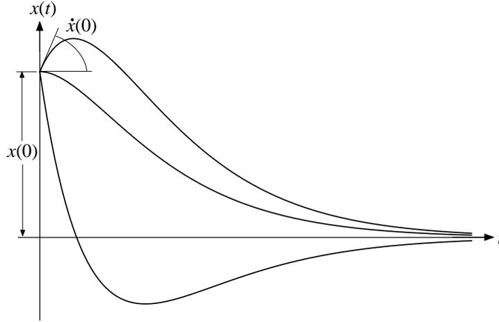
**Fig.2.2.4** Free vibration response of a critically damped system
