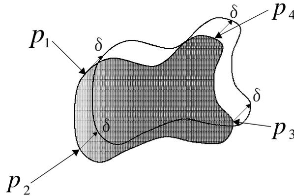
**Fig.2.5.1** Virtual displacement of a body
