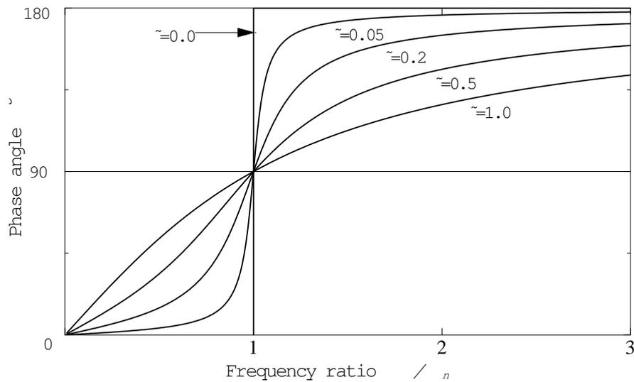
**Fig.2.3.3** Phase angle  $\theta$  with damping ratio  $\zeta$  and frequency ratio  $r_n$
