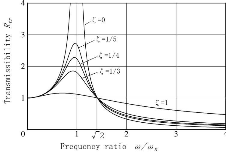
Fig.2.3.7 Vibration transmissibility ratio
