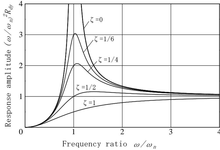
**Fig.2.3.5** Response of seismometer to harmonic base displacement
