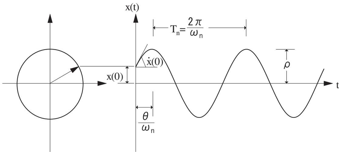
Fig.2.2.2 Undamped free-vibration response
