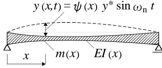
**Fig.2.6.2** Vibration of a nonuniform simple beam
