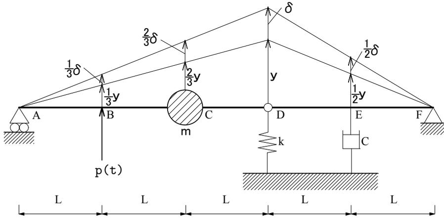
Fig.2.5.3 Virtual displacements of the system
