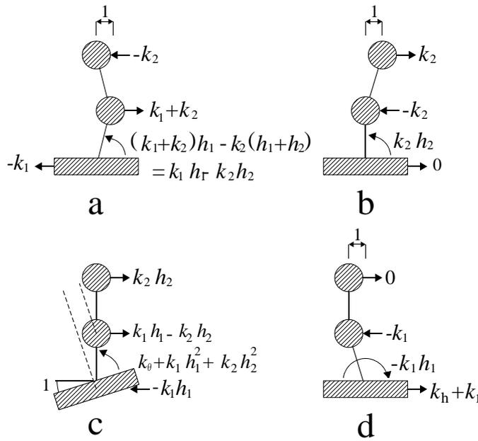
Fig.3.1.3 Elements of stiffness matrix
