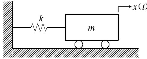
**Fig.2.6.1** Free vibration of an undamped spring-mass system
