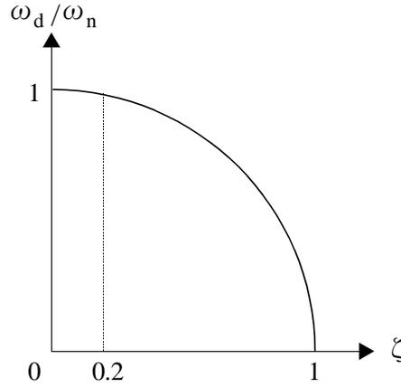
**Fig.2.2.5** Relationship between the ratio  $\omega_d/\omega_n$  and  $\zeta$
