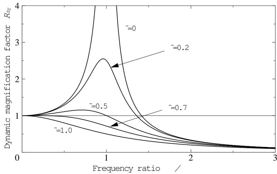
**Fig.2.3.2** Dynamic magnification factor  $R_{dy}$  with damping ratio  $\zeta$  and frequency ratio  $r_n$
