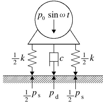
**Fig.2.3.6** Vibration isolation system
