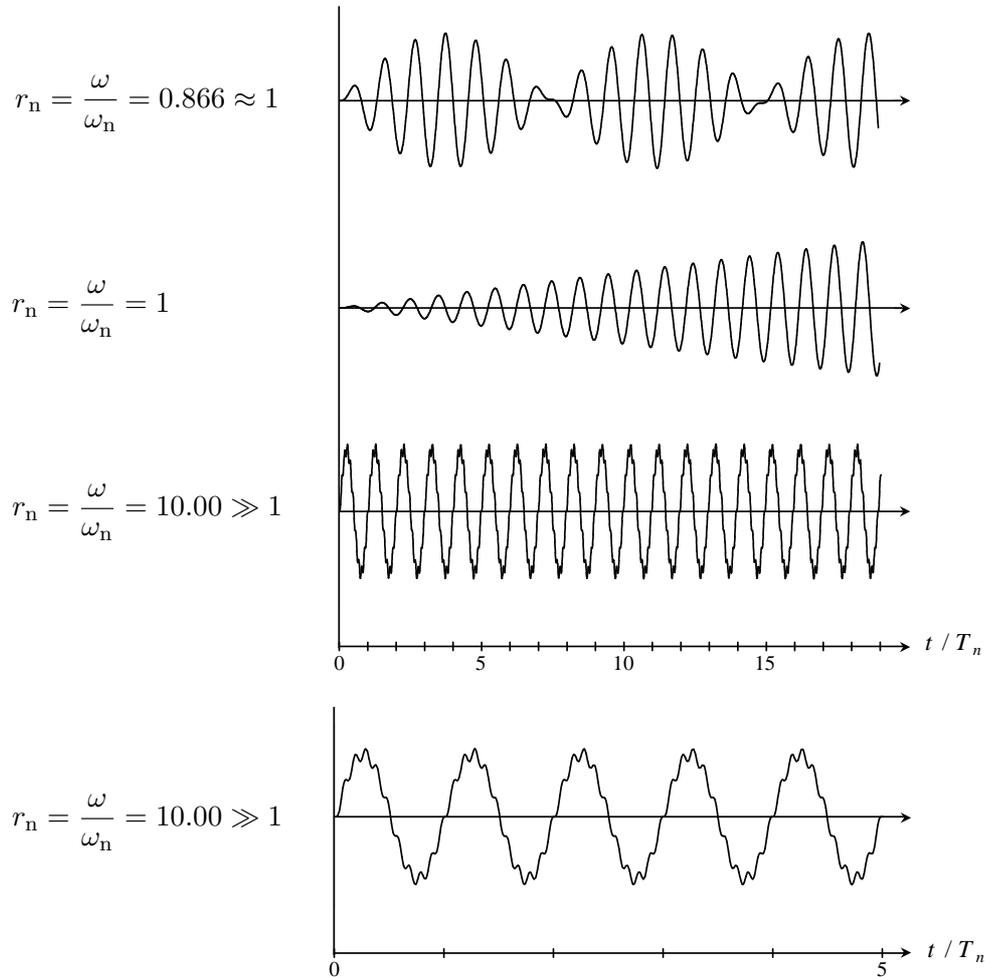
**Fig.2.3.1** Response of undamped systems to harmonic loading
