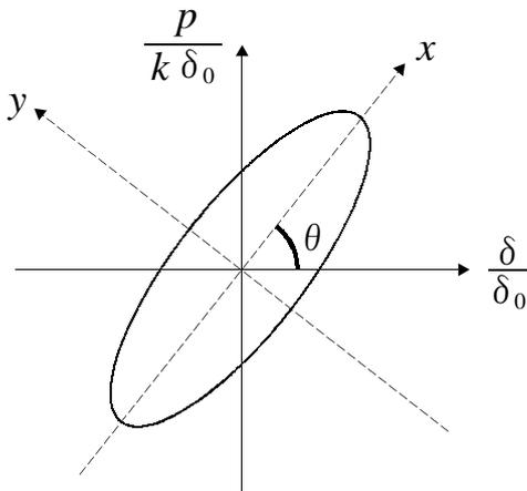
**Fig.3.5.2** Ellipse representing force and deformation relationship
